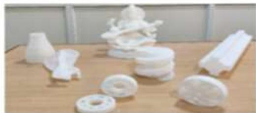
**Components manufactured using FDM**
