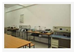
The Physics Laboratory is equipped with Band Gap Measurement kits, Hall Effect kits, LED Radiation pattern kits, V-I Power Curve Of Solar kits, Sound Intensity decibel kits, Velocity Measurement Ultrasonic Kits, Elasticity using Young's modulus kits.
